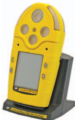
Optional rechargeable battery and slip-in cradle charger
